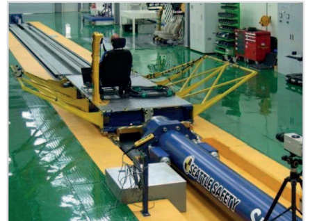
The test sled carrying the crash test dummy is propelled by compressed air.
